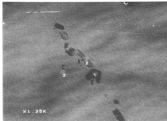
Figure 2 SEM photograph of the solution-treated alloy.
